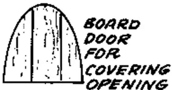
FIGURE 3. TIGHT FITTING WOODEN OR METAL COVERS ARE USED TO COVER DOOR OPENING AND SMOKE HOLE.
