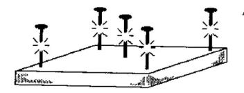
Make the top of the jig with the longer piece of wire. Bend the wire around the nails as described above. You will have some left over. Bend this part into a hook to hang up the jig with. Take the wire off the frame and bend down the corners as Shown in Figure 3.
