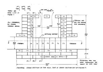
The firebox is a long rectangular chamber, fired from both ends so that the hot gases flow inward and upward (see Figure 1). Between and above the fires is the
