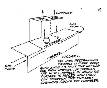
kiln chamber in which the pottery is placed. The hot gases rise through the chamber and go out the chimney opening at the top. Both the chamber and the firebox are surrounded by a layer of common brick. Figures 4 through 6 show how the bricks should be arranged. Note the staggering of joints in alternate courses.
